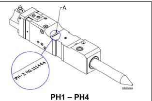
The serial number location is located left of center on face of body between hammer ports and retaining pin.
