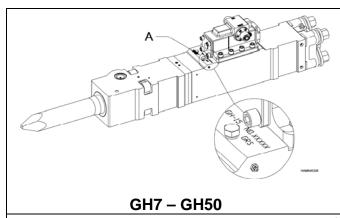
A The serial number location is right of center on the body above the autolube port.
