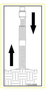
When the tool is not in contact with the material to be broken, the energy of the compression waves has nowhere to go and therefore, returns totally in the chisel as tensile waves. This is referred to as a "blank hammer blow".
