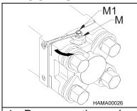
1. Remove the charge valve (M1) from the charge valve (M). Do not remove the charge valve assembly!
