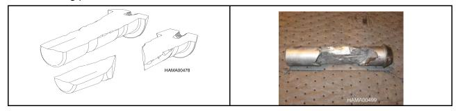
3. If chipping (16) is found at the top of the tool, replace the tool. If neglected, the piston impact surface will be damaged (AM is normal, AL needs to be replaced).
