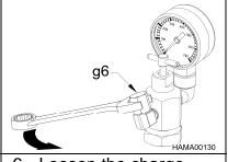
6. Loosen the charge adapter cap (g6) VERY SLOWLY! The gas pressure will gradually decrease to zero. When it gets to zero, remove the cap.
