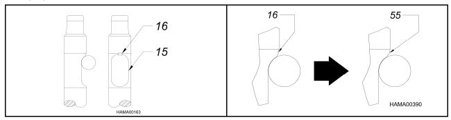
2A. Excessive blank hammering can cause retaining pin breakage/failure. Replace retaining pin.
