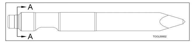
For warranted tool failures, a prorated credit, up to 80% maximum, will be issued for tools with tip wear greater than 50 mm on chisel and moil points, or 30 mm on blunt end tools. Note: Parts replaced under warranty become the property of NPK.
