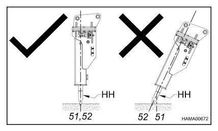
Keep the boom direction of force (51) in the same direction the tool is penetrating. Use the boom cylinder to preload the hammer (apply down force), and use the bucket and stick cylinders for alignment. Keep the tool tangent to the arc of the boom (54).
