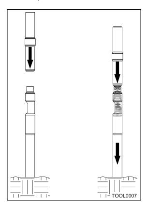
Impact force is transmitted as stress waves through the tool.
