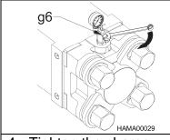
4. Tighten the charge adapter cap (g6).
