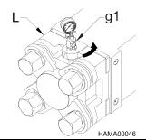
7. Remove the charge adapter (g1) from the gas charge valve on the hammer gas head (L), then, reinstall the charge valve cap.
