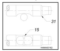
2. Excessive blank hammering will cause chipping (16) in the retaining pin contact area (15). If neglected, the chipping may reduce the life of the tool. Dress with a grinder (55).
