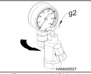
2. Turn the NPK charge adapter T-handle (g2) to a full counterclockwise position.
