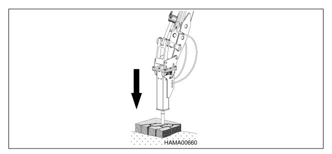
APPLY DOWNFORCE TO PUSH TOOL UP INTO HAMMER
