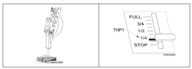
3. Place the hammer firmly against the material to be broken (see "PRELOAD THE TOOL BEFORE STARTING"). Operate the hammer in a vertical position for approximately 10 minutes at one-half (THP2) engine speed. Increase the engine speed to three-quarters (THP3) and continue operating at this speed for another 10 to 20 minutes. Increase to full engine speed (THP4). Maintain vertical position for the duration of the operation.
