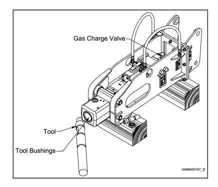
Install hydraulic hoses to the hammer valve and to plugs provided on the hammer bracket. Verify all attaching hardware is torqued to NPK specifications. Bolt torque specifications are listed in the Operators Manual.
