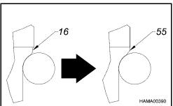
3. Excessive blank hammering can cause retaining pin breakage/failure. Replace retaining pin.
