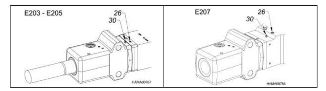
If an Auto Lube System is not used, you can grease the unit manually through the grease fitting (30).
