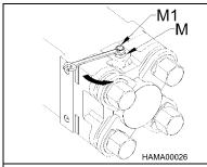
1. Remove the charge valve cap (M1) from the charge valve (M). Do not remove the charge valve assembly!
