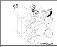
4. Tighten the charge adapter cap (g6).
