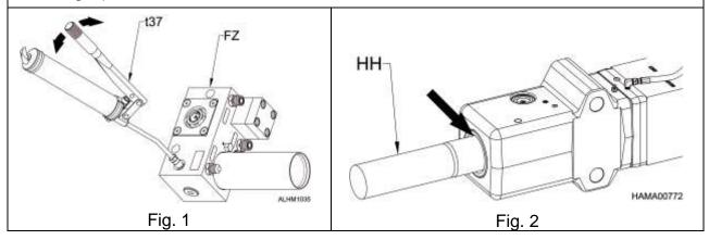
NOTE: If the Auto Lube unit has run out of grease, the above procedure should be used to purge all air out of the grease line before using the hammer. Failure to do this will result in an intermittent supply of grease to the hammer.
