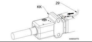
8. Pump twenty more shots of grease, using a grease gun (t37) or power greaser, into the pump assembly (FZ). This will prime the hammer tool cavity and pre-lube the tool (HH). Look for grease coming out around the tool at the tool bushing (see arrow in Fig. 2).
