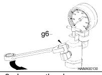
6. Loosen the charge adapter cap (g6)
