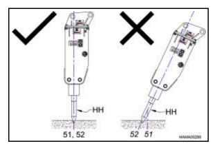
Keep the boom direction of force (51) in the same direction the tool is penetrating. Use the boom cylinder to preload the hammer (apply down force) and use the bucket and stick cylinders for alignment. Keep the tool tangent to the arc of the boom (54).
