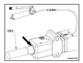
4. Grease hammer at least once an hour. See "CORRECT FUNCTION OF GREASING AND GREASE INTERVALS" for a more exact greasing procedure.
