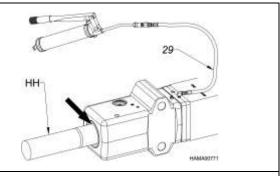
11. Remove the hose fill adapter (a13) and re-connect the grease line (29) to the Auto Lube pump (FZ).
