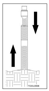
The compression waves and the tensile waves travel in a complex manner in the tool during hammer operation. While these waves are gradually being attenuated by the internal friction of the tool and by the friction between the tool and the tool holder bushings, the next impact strikes the tool. Excessively heavy contact between the tool and tool bushings causes uneven stress concentrations. This leads to premature tool failure, as seen in later sections of this manual.
