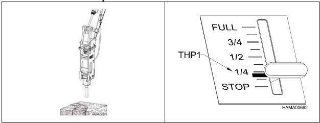
3. Place hammer firmly against the material to be broken (see "PRELOAD THE TOOL BEFORE STARTING"). Operate the hammer in a vertical position for approximately 10 minutes at one-half (THP2) engine speed. Increase engine speed to three-quarters (THP3) and continue operating at this speed for another 10 to 20 minutes. Increase to full engine speed (THP4). Maintain vertical position for the duration of the operation.
