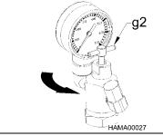
Turn the NPK charge adapter T-handle (g2) to a full counterclockwise position.
