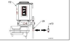
NOTE: If the Auto Lube unit has run out of grease, the above procedure should be used to purge all air out of the grease line before using the hammer. Failure to do this will result in an intermittent supply of grease to the hammer.
