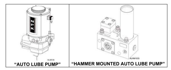
The NPK Auto Lube Systems are designed to automatically provide a continuous supply of grease to the hammer tool and tool bushing, increasing tool and tool bushing life by reducing wear. The Auto Lube pumps are capable of pumping EP2 grease in cold weather. The pump output is adjustable according to the replacements of the hammer model and to compensate for tool bushing wear.
