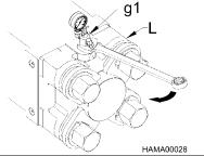
Install the NPK charge adapter (g1) onto the hammer charge valve located on the hammer gas head (L).
