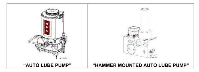
The NPK Auto Lube Systems are designed to automatically provide a continuous supply of grease to the hammer tool and tool bushing, increasing tool and tool bushing life by reducing wear. The Auto Lube pumps are capable of pumping EP2 grease in cold weather. The pump output is adjustable according to the replacements of the hammer model and to compensate for tool bushing wear.
