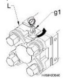
7. Remove the charge adapter (g1) from the gas charge valve on the hammer gas head (L), then, reinstall the charge valve cap.
