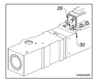
If an Auto Lube System is not used, you can grease the unit manually through the grease fitting (30).
