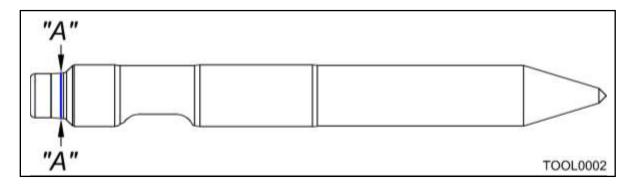
For warranted tool failures, a prorated credit, up to 80% maximum, will be issued for tools with tip wear greater than 50 mm on chisel and moil points, or 30 mm on blunt end tools. Note: Parts replaced under warranty become the property of NPK.
