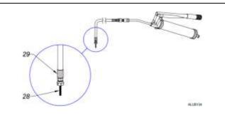
7. Re-attach the grease line (29) to the hammer assembly (KK).
