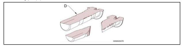
3. If chipping (16) is found at the top of the tool, replace the tool. If neglected, the piston impact surface will be damaged.
