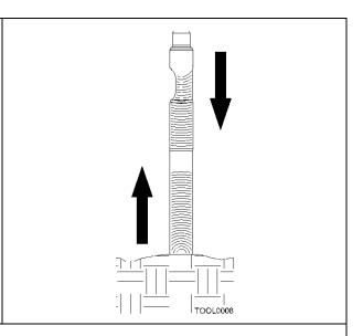
When the tool is not in contact with the material to be broken, the energy of the compression waves has nowhere to go and therefore, returns totally in the chisel as tensile waves. This is referred to as a "blank hammer blow", see page 31.
