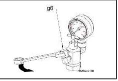
6. Loosen the charge adapter cap (g6) **VERY SLOWLY!**The gas pressure will gradually decrease to zero. When it gets to zero, remove the cap.
