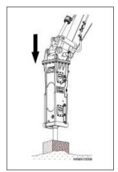
First, grease the hammer at the beginning of the job until grease comes out between the tool and the lower tool bushing. Run the hammer until the shank of the tool starts to look dry. This determines the time interval for the greasing of this particular hammer on this particular job. Typically, this is 1 to 4 hours. Also, note the amount of grease needed to re-grease the tool. This gives you the amount of grease and how
