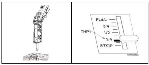
3. Place hammer firmly against material to be broken (see "PRELOAD THE TOOL BEFORE STARTING").
