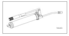
often it must be applied. An example would be that a particular hammer, on a particular job, requires half a tube of grease every 3 hours. This would be the greasing schedule you would set up. If this hammer was moved to another job, another grease schedule may have to be determined.
