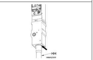
NOTE: If the Auto Lube unit has run out of grease, the above procedure should be used to purge all air out of the grease line (29) before using the hammer. Failure to do this will result in an intermittent supply of grease to the hammer.
