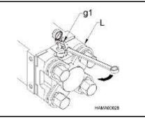
3. Install the NPK charge adapter (g1) onto the hammer charge valve located on the hammer gas head (L).
