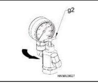
charge 2. Turn the NPK charge om the adapter T-handle (g2) to a full counterclockwise charge position.
