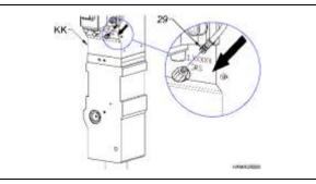
8. Pump twenty more shots of grease, using the grease gun (t37) or power greaser, into the pump assembly (FZ). This will prime the hammer tool cavity and pre-lube the tool (HH). Look for grease coming out around the tool at the tool bushing (see arrow).
