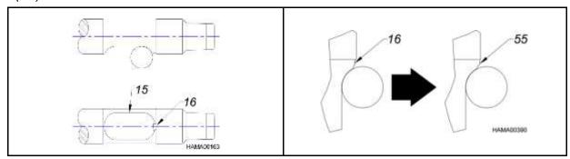
2A. Excessive blank hammering can cause retaining pin breakage/failure. Replace retaining pin (D).
