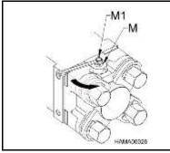
1. Remove the charge valve cap (M1) from the charge valve (M). **Do** not remove the charge valve assembly!
