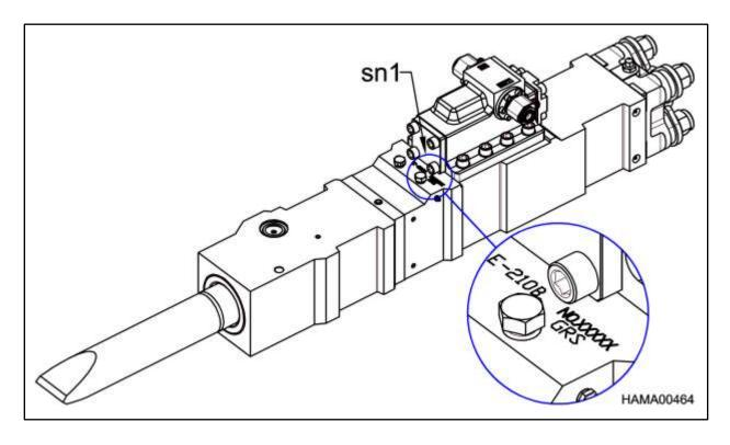
The serial number location (sn1) is right of center on the body above the Auto Lube port.
