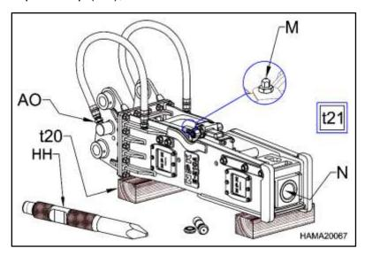
If the NPK HYDRAULIC HAMMER is not to be used for a long period of time (months), it is recommended the gas pressure be discharged at the charge valve (M). The tool (HH) should be removed, and the piston (N) pushed all the way in. Be sure the hydraulic hoses are plugged and grease the exposed end of the piston (N). Grease and reinstall the tool (HH). Cover with a waterproof tarp (t21), not shown.
