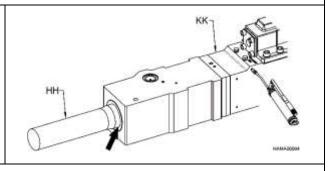
4. Grease hammer at least once an hour. See "CORRECT FUNCTION OF GREASING AND GREASE INTERVALS" for a more exact greasing procedure.
