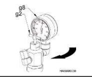
5. Turn the T-handle (g2) clockwise. As the T-handle is screwed in, a resistance is encountered. By turning the T-handle, the nitrogen gas pressure will be indicated on the pressure gauge (g8). Stop turning the T-handle when the gauge reads pressure. **Do not overtighten!**
