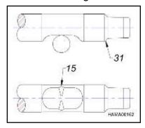
2. Excessive blank hammering will cause chipping (16) in the retaining pin contact area (15). If neglected, the chipping may reduce the life of the tool. Dress with a grinder (55).
