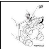
4. Tighten the charge adapter cap (g6).
