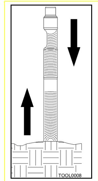
When the tool is not in contact with the material to be broken, the energy of the compression waves has nowhere to go and therefore, returns totally in the chisel as tensile waves. This is referred to as a “blank hammer blow”.
