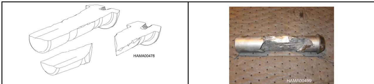
3. If chipping (16) is found at the top of the tool, replace the tool. If neglected, the piston impact surface will be damaged (AM is normal, AL needs to be replaced).
