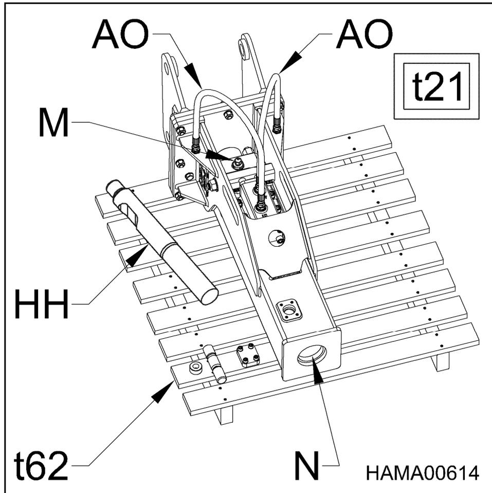
If the NPK HYDRAULIC HAMMER is not to be used for a long period of time (months), it is recommended the gas pressure be discharged (M). The tool (HH) should be removed, and the piston (N) pushed all the way in. Be sure the hydraulic hoses are plugged and grease the exposed end of the piston (N). Grease and reinstall the tool (HH). Cover with a waterproof tarp (t21), not shown.
