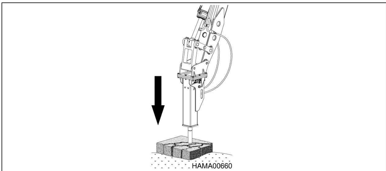
APPLY DOWNFORCE TO PUSH TOOL UP INTO HAMMER
