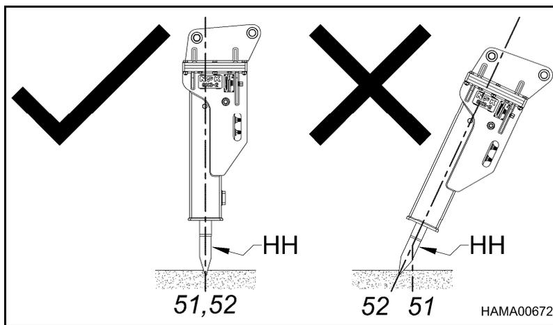
Keep the boom direction of force (51) in the same direction the tool is penetrating. Use the boom cylinder to preload the hammer (apply down force), and use the bucket and stick cylinders for alignment. Keep the tool tangent to the arc of the boom (54).
