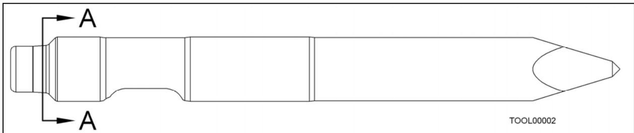
***For warranted tool failures, a prorated credit, up to 80% maximum, will be issued for tools with tip wear greater than 50 mm on chisel andmoil points, or 30 mm on blunt end tools. Note: Parts replaced under warranty become the property of NPK.***
