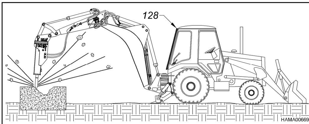
**DO NOT OPERATE THE HAMMER WITHOUT AN IMPACT RESISTANT CAB WINDOW OR SHIELD (128) IN PLACE**
