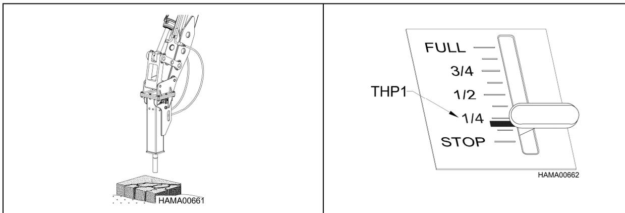
3. **Place the hammer firmly against the material to be broken (see “PRELOAD THE TOOL BEFORE STARTING”).** Operate the hammer in a vertical position for approximately 10 minutes at one-half (THP2) engine speed. Increase the engine speed to three-quarters (THP3) and continue operating at this speed for another 10 to 20 minutes. Increase to full engine speed (THP4). Maintain vertical position for the duration of the operation.
