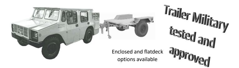
Frame, body & enclosure are composed of coated aluminum alloy with reinforced high strength steel drawbar & sling/tie-down point making trailers extremely durable & corrosion resistant while minimizing weight.
