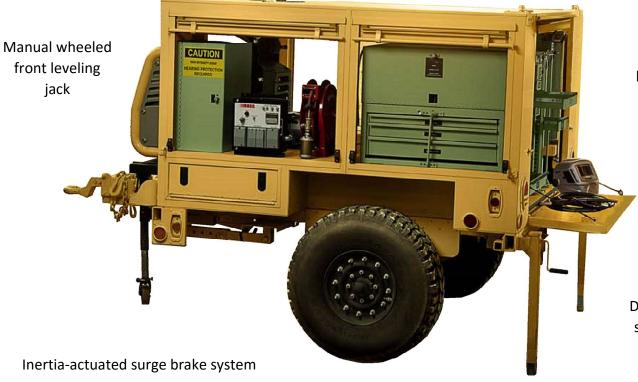
Weather resistant locking roll up doors secure all access openings
