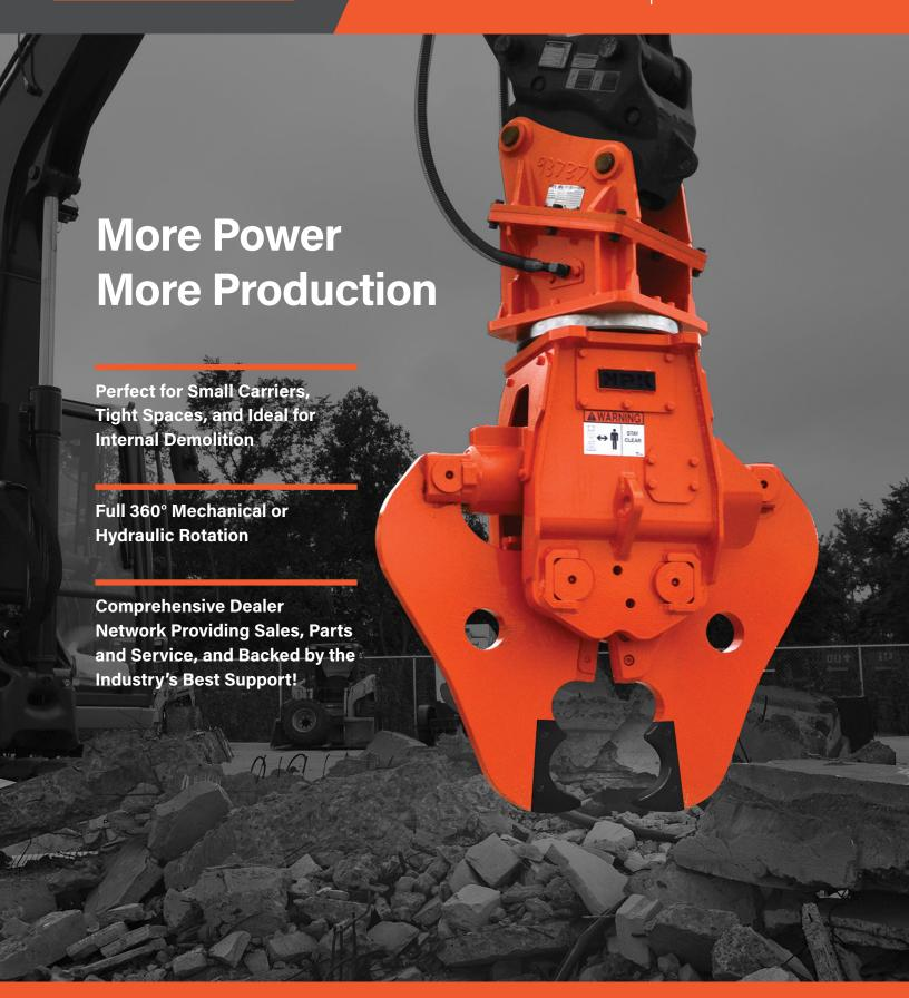
NPK's Concrete Crushers are designed to effectively handle any primary and/or secondary demolition and recycling operation. NPK Crushers easily cut through reinforced concrete and light steel structures allowing material to be separated and recycled while simultaneously permitting easier handling of material.
